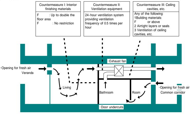
\* Only area size restrictions of interior finishing materials (Countermeasure I) apply to houses of traditional Japanese construction ("shinkabe" (earth-plaster wall) construction, with no plywood, etc., used on ceilings and floors).
