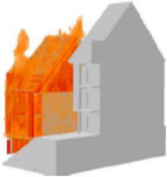
Third phase: widespread conflagration and Spread to the nearby "E" Building
