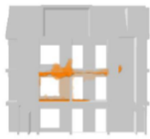
First phase: balcony fire + façade then apartment fire
